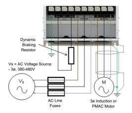
Note: Power terminals shown are for Frame 7. Although other frames may vary slightly in appearance and sequence, their terminal designations and functionality are identical.
