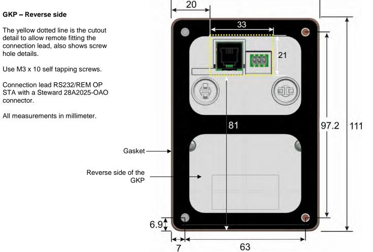
detail to allow remote fitting the connection lead, also shows screw hole details.
